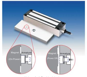
Unique Anti-Residual design When there is no power, there will be no holding force, and the push-off button will pop out immediately, to release the Electromagnetic Lock and the Armature Plate for no residual magnetism.
